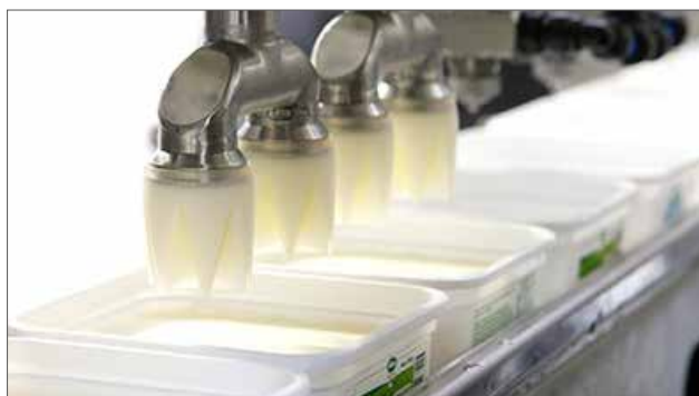
Cup filling station with drip free nozzles.
